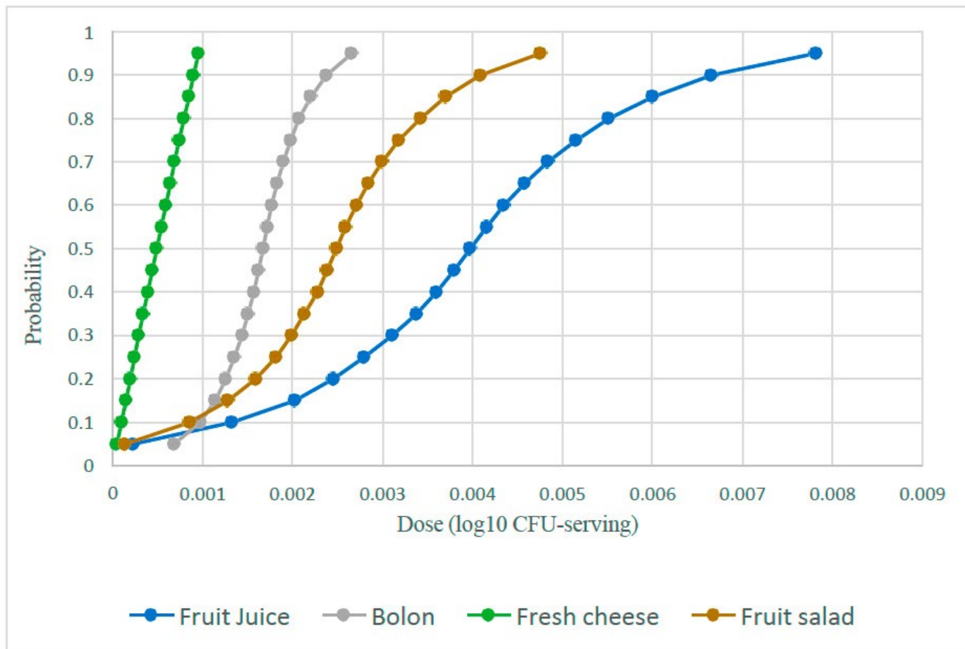
Figure 3: Dose-response graph for Listeria monocytogenes in 4 types of food evaluated in Guayaquil, Quito, Cuenca
